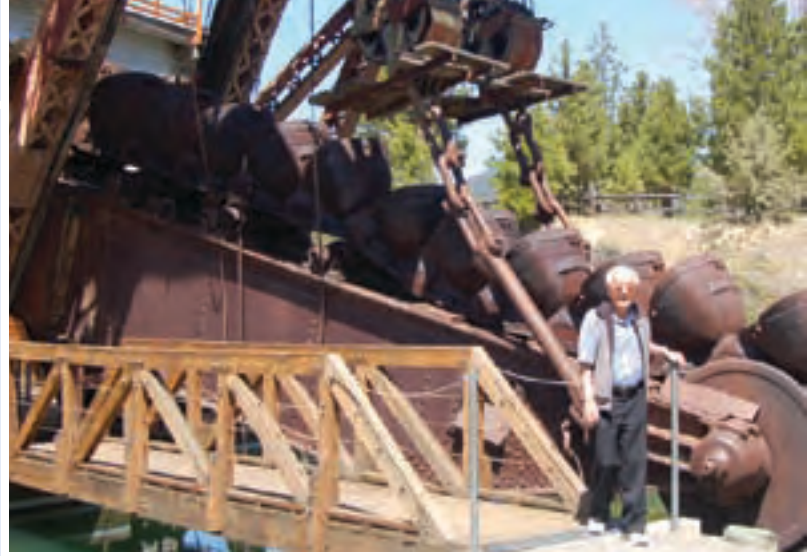
Dr. Tanaka stands in front of the dredge bucket line. Each bucket weighs one ton and holds about four square yards of material.
